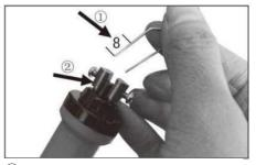
①The feet of the pen point shall be inserted into the copper binding post for more than 8 mm.
