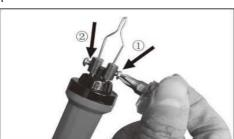
①Tighten the screw with the screwdriver and tighten the feet of the pen point! It must be tightly closed; otherwise, the pen point won't be heated or its heating is abnormal or even sparks.
