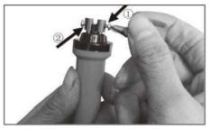
①Here the top screw needs to exit more than 4 mm, and the screw needs to exit this distance and inserts into the pen point.
